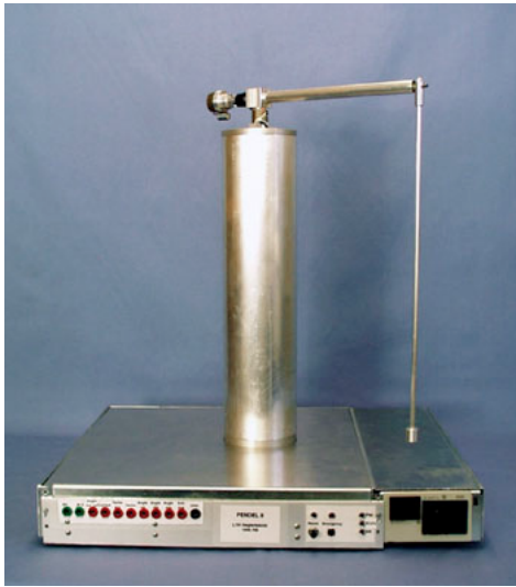
Figure 6.11. The Furuta pendulum.
